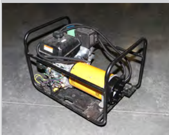
A Winco generator (left) can be distinguished by its yellow stator housing, whereas the Baldor has either a black or red stator housing (right).
