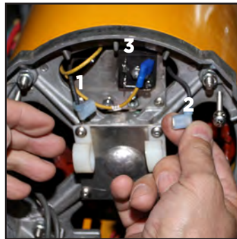
Remove blue negative (1) and positive (2) flag connectors from bridge (3).
