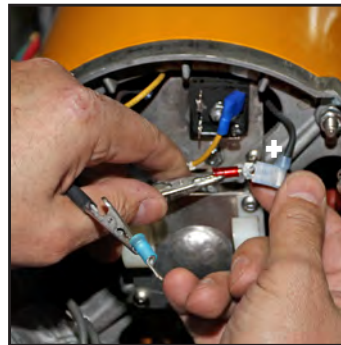
Connect the positive lead from battery to the positive flag connector.
