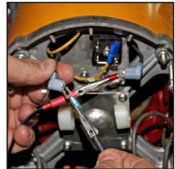
Momentarily touch the negative lead from the battery to the negative flag connector - just long enough to create an arc.
